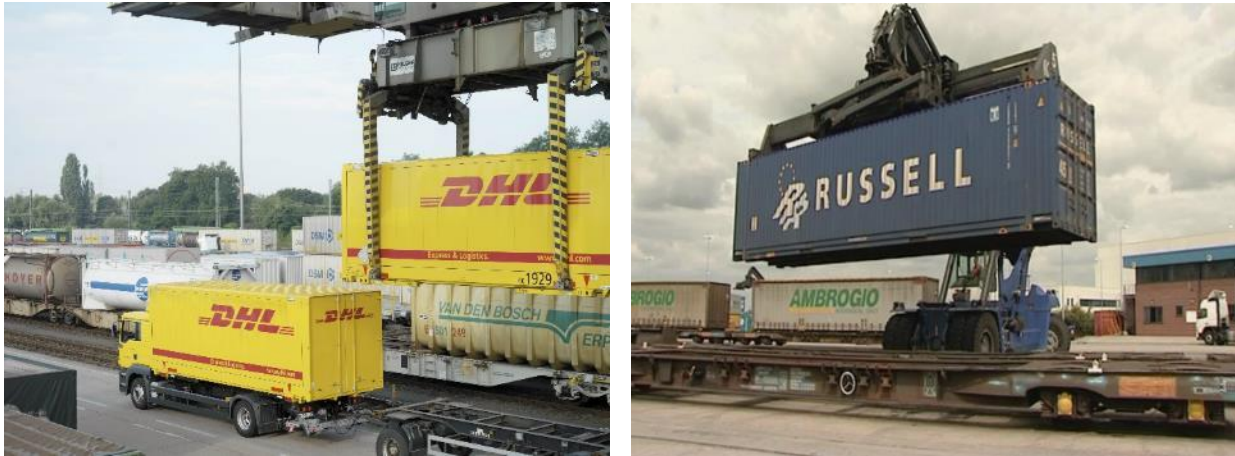
Figure 3 Overhead gantry crane (left), reachstacker (right)
