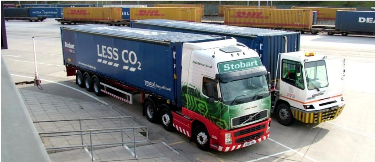
Figure 4 Containers with road tractor unit (left) and tugmaster (right)
